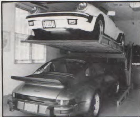
Harding-AFG CAR LIFT has an exclusive feature that allows us to stack two cars totaling in height more than the ceiling height.
